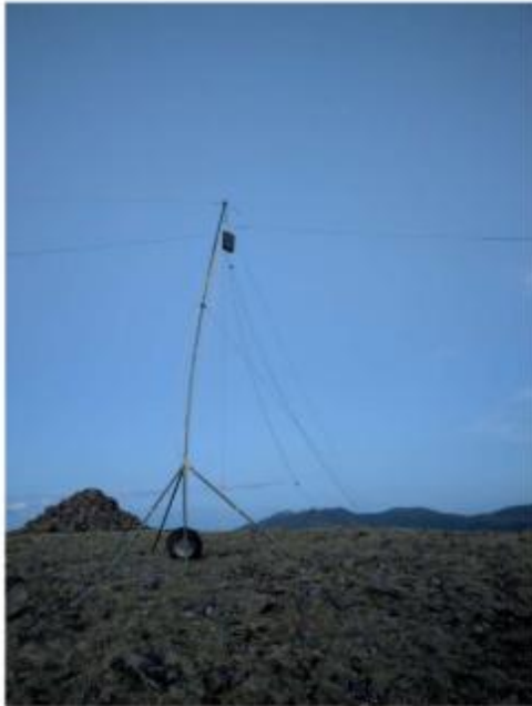
Figure 1: 24' of mast, SGC 230 tuner, 43'x2 doublet, along with a 20m coaxial dipole at a right angle
