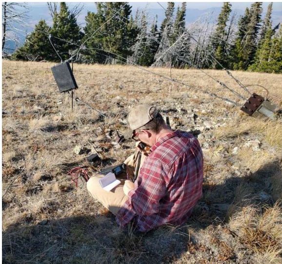
KE7VUX uses the tower guy wires as his HF antenna. Notice the tuner hanging from the guys!
